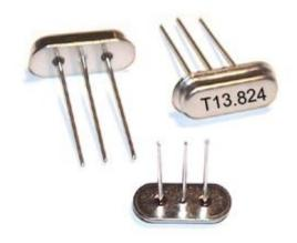
Package Height 3.5 mm max, 2.5~3.5 mm available Wave Soldering Temperature: 265°C max Highly stable and reliable crystal unit with a metallic package 3 Pin with ground pin
